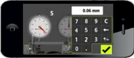
Enter the horizontal offset values on stationary (S) and moveable (M).
