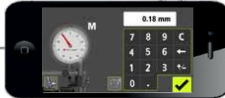
Rotate the dials to 12.00. Enter the vertical offset values on stationary (S) and moveable (M).
