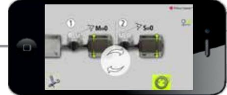
Do the final corrections Adjust moveable machine until dials read zero! Remeasure to check your work!
